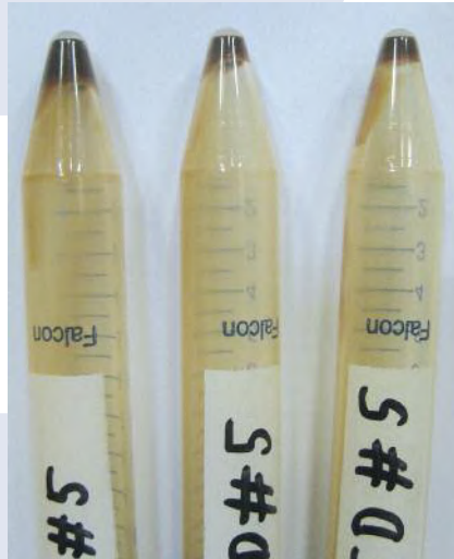
Spin tests to evaluate the volumetric composition of different extracts as well as consistency of their solids
