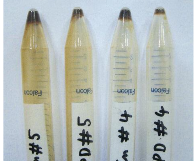
Spin tests to evaluate the volumetric composition of different extracts as well as consistency of their solids
