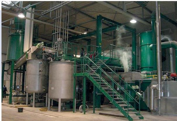
FLOTTWEG SORTICANTER® system for the recovery of polyolefins from mixed plastics at a German company
